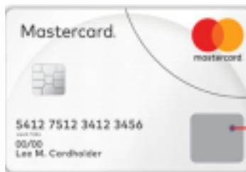
Embedded fingerprint sensor to capture and match the cardholder's fingerprint to the digital fingerprint image stored on the card.
